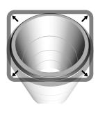
Lubrication of the socket or spigot is not required. Centre the joint and assemble. The position of the seal in the final mahole joint is shown.
