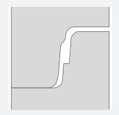
fully closed to ensure the lubricat stays in place. During installation the thin mantle slides over the body of the seal. This design permits installation with very low force, as there is no friction between rubber and concrete.
