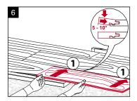
Pull the vinyl installation aid out (Figure 7) and position it or, when installing large formats with a strip, pull it forward to install the following plank. It, like all the rest, is then clicked in place in the same way on the end side
