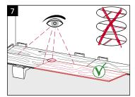
Alternatively, from the second row onwards you can use the following installation technique:
