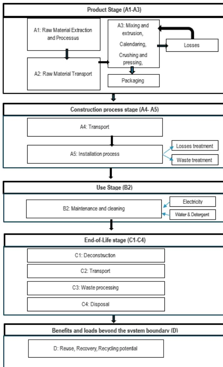
Process flow diagram of the product system, divided into the life-cycle stages and modules (or other division of the product life cycle, if defined in the PCR), showing the main processes included and the system boundary of the LCA. The diagram shall make it clear when the end-of-waste state is reached for main input flows of reused/recycled materials and recovered energy, and for output flows of reused/recycled materials and recovered energy exiting the end-of-life stage.
