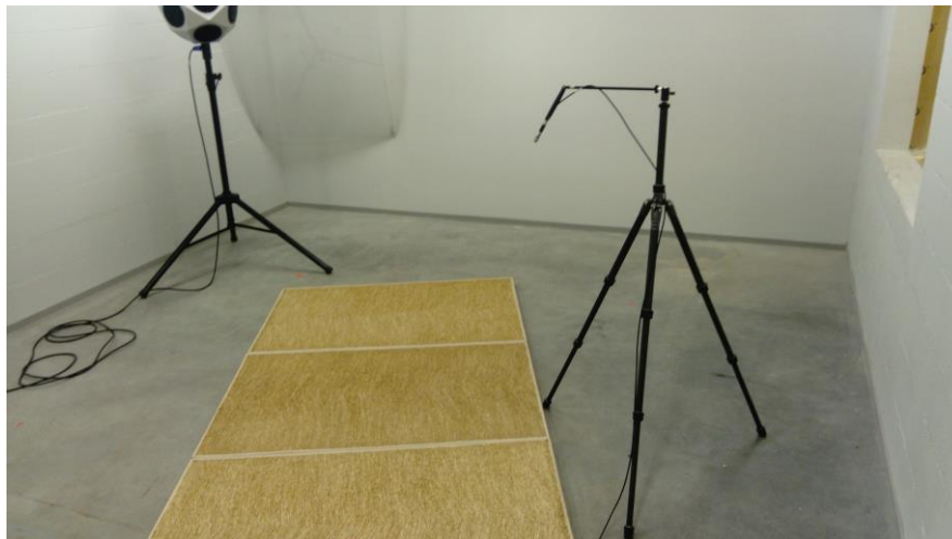
Figure A2-1. An example of installation of test object in TalTech acoustics laboratory's reverberation room. Omnidirectional acoustic source (loudspeaker) and tripod mounted condenser microphone are exhibited in the background and foreground accordingly.
