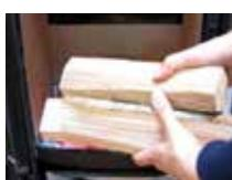
The stove door should normally be opened gently the first 2-3 cm, then you should wait until the pressure has equalised before opening the door all the way. This technique will prevent smoke from getting out, particularly when there is a poor draught.
