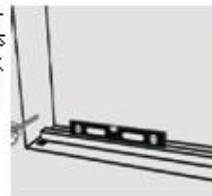
**EN:** Decide and mark the position of the frame in relation to the inner and outer wall.
