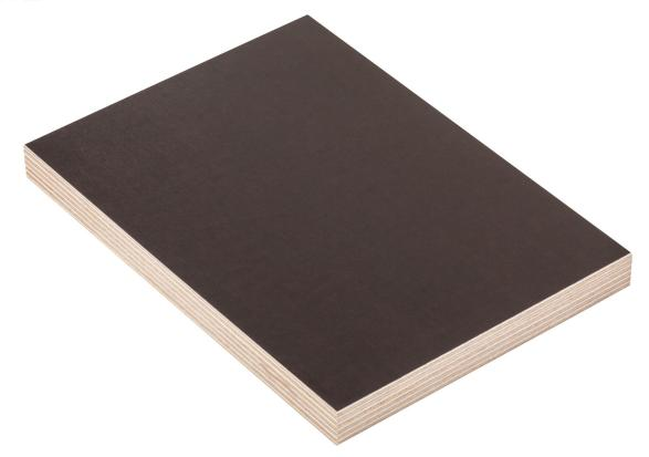
Metsä Wood Form is birch plywood, in which both sides are overlaid with phenol film and the edges are sealed. Form plywood is an ideal formwork panel for smooth surfaced concrete elements. It can also be used as a multipurpose, maintenance-free panel for various other uses. Metsä Wood Form is available in sizes standard, L, XL and KingSize.
