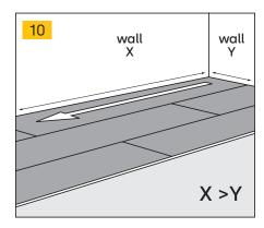
**LAYOUT:** We recommend to install the floor towards the light or in the direction of the longest wall. (Pic. 9 & 10)
