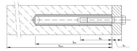
$t_{\text{fix}}$  = thickness of fixture
