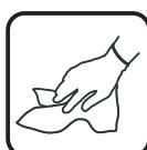
Clean the surfaces with a soft brush or cloth. Do not use water, aggressive solvents or sharp objects for cleaning to avoid damaging.
