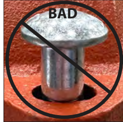
OVAL NECK OF BOLT NOT SEATED PROPERLY
