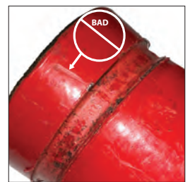
BAD PIPE END CONTAINS A LARGE INDENTATION IN THE PAINT ON THE "A" DIMENSION
