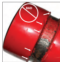
BAD PIPE END CONTAINS PUCKERED/ WAVY PAINT ON THE "A" DIMENSION
