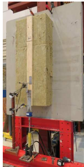
Pre-cast concrete test setup
