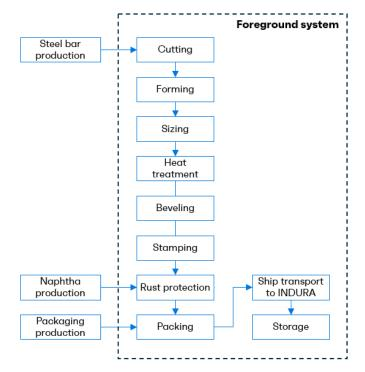
The product stages (A1 and A3) for butt welded fittings can be seen above.
