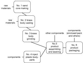
No. 1: The sand core for the base body is made.
