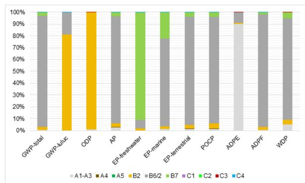
The dominance analysis shows that module A1-A3 in particular is the dominant life cycle stage in regard to GWPtotal (2.20 kg CO2-eq.). This is mainly caused by the provision of brass for the production of the basic sets at the production site (0.64 kg CO2-eq.) The end-of-life stage (module C1-C4) has a noteworthy influence on the indicator GWPtotal and also on AP, EP, POCP and WDP. Here, these indicators are each influenced primarily by the thermal treatment of plastics.
