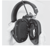
4. When placing the new ear pad, the halfround shape should be on top.
