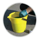
**1.** Mix drain dye with water. 1 teaspoon of drain dye to approx 10 litres of clean water.
