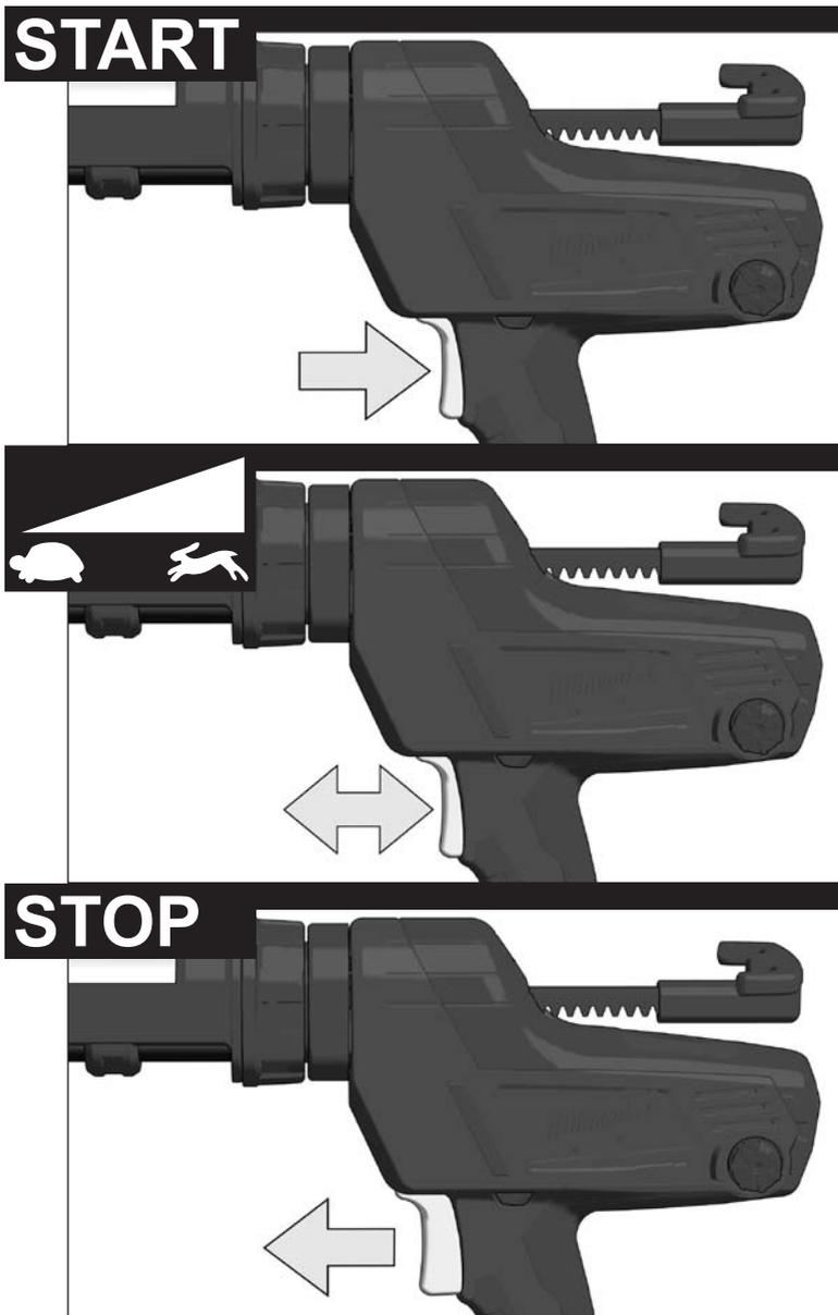
When the trigger is released, the motor will run for a short time to release the rod. This prevents a drip. When a tube is emptied, the motor will run for a short time to release the rod.
