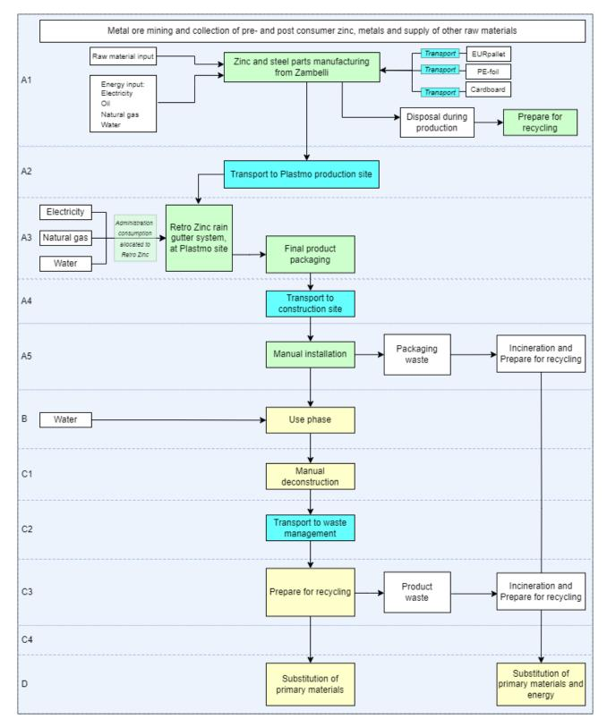
System boundaries of the entire life cycle of the Retro Zinc Rain Gutter System divided into the relevant modules. All modules are covered in this LCA. Color coding; White: inputs & outputs; blue: transport; green: A modules; yellow: B-D modules.
