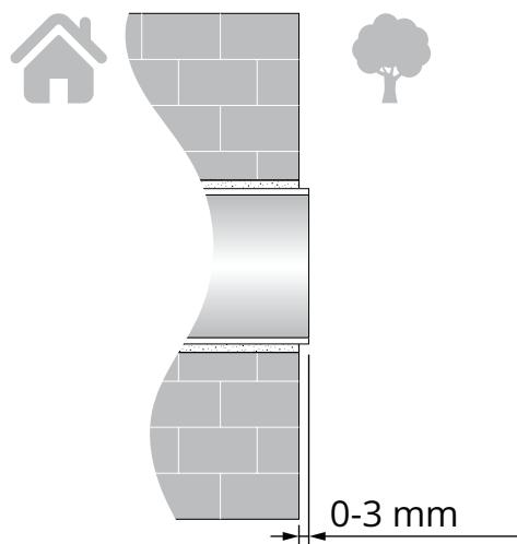
2. Mark the fastening holes for the outer ventilation hood and drill 4 holes, 50 mm deep to suit the expansion anchors. Use the back wall of the ventilation hood to facilitate the marking.
