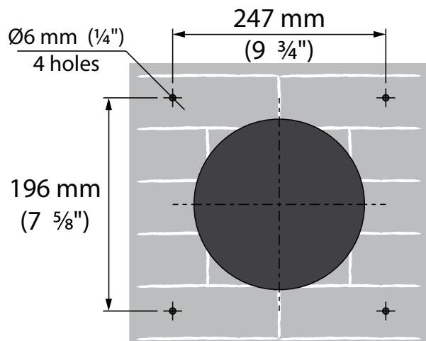
3. Insert the supplied expansion anchors 6x40 into the holes.
