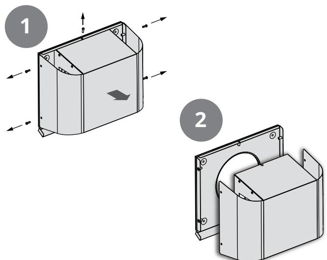
4. Fix the back wall of the ventilation hood on the wall using the supplied screws 4x40.
