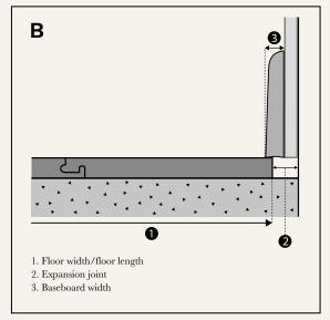
Ensure that the floor can move freely beneath the wall panels.
