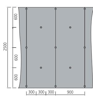
Montering: Full overflate liming og dowelling for BA12,5; BA20; BA30; BA50 mm.
