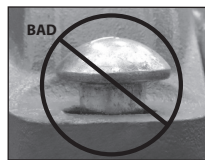
OVAL NECK OF BOLT NOT SEATED PROPERLY
