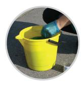
**1.** Mix drain dye with water. 1 teaspoon of drain dye to approx 10 litres of clean water.
