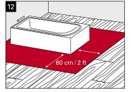
Vinyl flooring with HDF core board must not be installed in areas where water can splash on the floor (Figure 12). Standing water penetrates the HDF core board via the edges and causes permanent damage.
