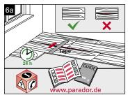
Removal and possible repositioning is possible shortly after installation. Generally, the plank elements must be pressed properly down into the adhesive. Rolling with a pressure roller (weight 50 kg) is necessary for whole-area gluing with the substrate as well as for installation on the self-adhesive underlay (Figure 7). The adhesive has dried completely after approximately 24 hours – in case of Parador Stick-Protect directly after rolling.
