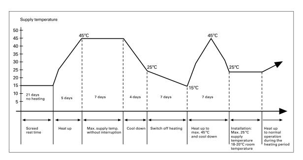
Please bear in mind: The surface temperature of the design flooring should ideally not exceed 25  $^{\circ}$ C (max. 28  $^{\circ}$ C).
