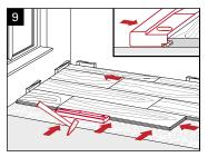
Disassembly instructions for vinyl flooring with SPC core board, vinyl flooring made of solid material and Modular ONE Hydron
