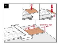
Note: Please precisely check the position (long and short edge, parallelism, perpendicularity) of planks without click geometry during installation (Figure 6). If there are slight gaps during installation, these can simply be pulled together with an adhesive tape. The adhesive tape can be removed once the surface has hardened (Fig 6a).
