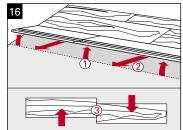
Disassembly instructions for vinyl flooring with HDF core board and Modular ONE
