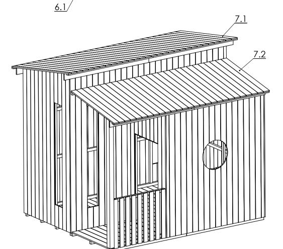
The last roof boards must be cut in right width
