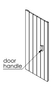
Connect the door handle from inside using 2x30mm screws
