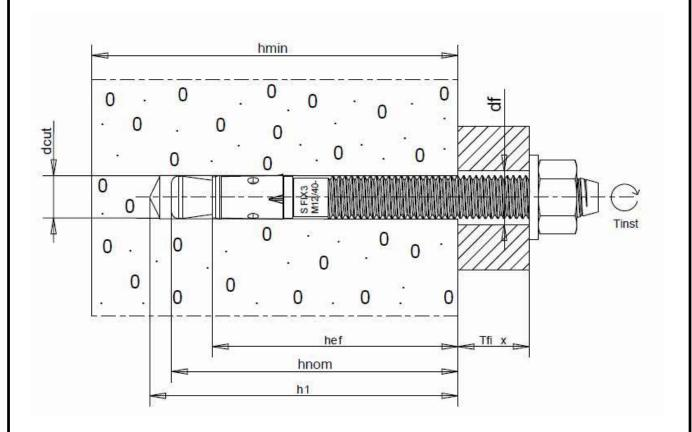
h<sub>ef</sub>: Effective anchorage depth h<sub>nom</sub>: Installation depth h<sub>1</sub>: Depth of drilled hole to deepest point
