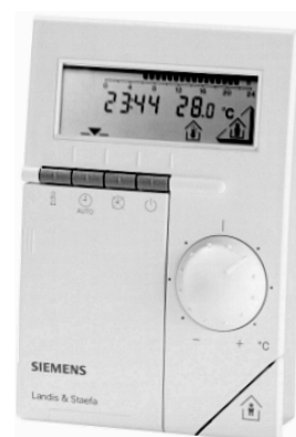
Room unit QAW70 with room sensor, time switch, setpoint adjustment, knob for room temperature setpoint readjustments and economy button
