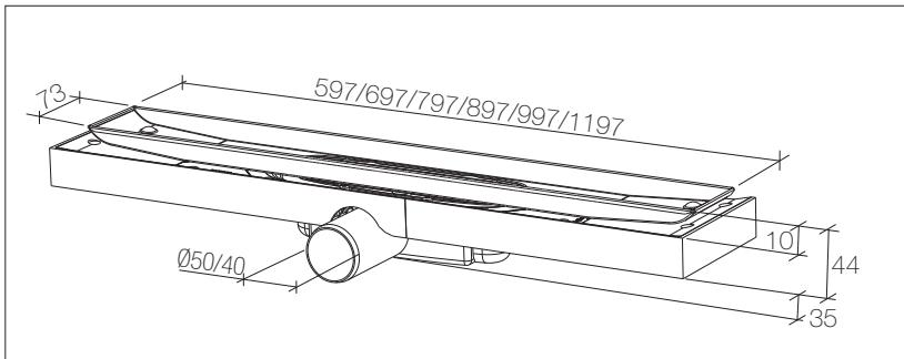
\*Kun for innstøping. Only for concrete joists.
