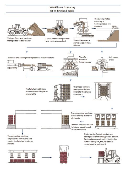
The flow diagram conforms with the requirements in the modular approach and shows the production phase A3 for Gandrup Teglværk with the exception that "handcut" is not used. The remaining phases are described below.
