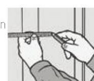
**UK:** Decide and mark the position of the frame in relation to the inner and outer wall.
