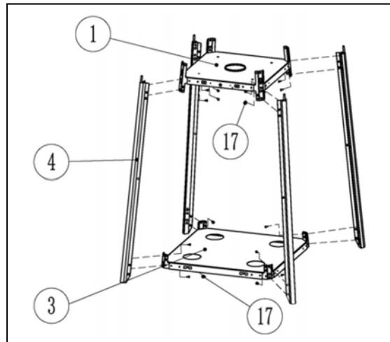
**21. Connect and fix the 4 lower supports(4) to bottom plate(3) and middle plate(1) by the screws(17)**
