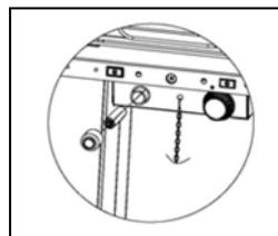
**1. Ensure that the control knob is OFF. Slowly open the gas cylinder valve.**
