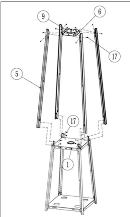
**22. Connect 4 upper supports (5) to the lower supports (4) and fixed by screws(17), then fix the upper plate(6) to 4 upper supports(5) by screws(17).**
