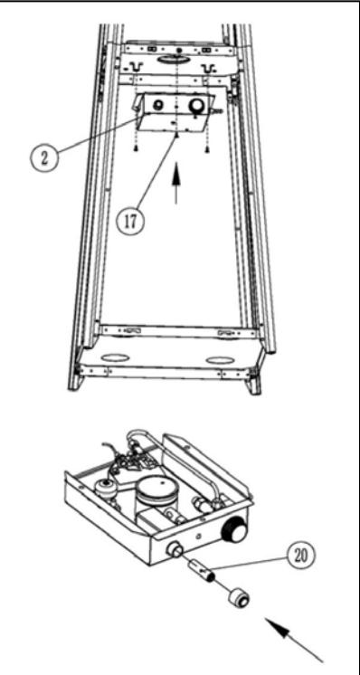
**24. Install a AA battery(20) into the control box, then, fix the control box(2) underneath the middle plate(1) by screws (17)**
