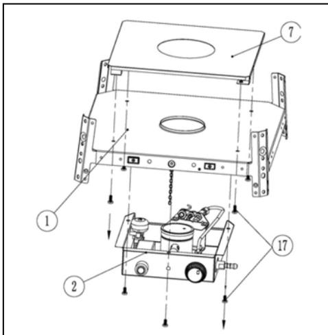
**20. Take the control box(2) and the plate cover(7) out off the middle plate(1) by unscrew the screws(17)**
