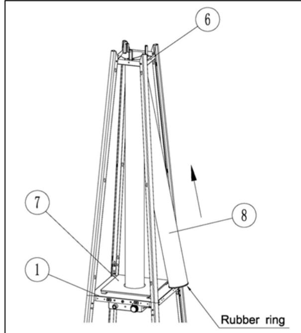
**25. Carefully put the glass tube(8) up through the center hole in the upper plate(6), Make sure the rubber ring is attached on the lower end of the glass tube(8). Move and sit the glass tube(8) through the hole of the plate cover(7) on the middle plate(1), check and ensure that the glass tube(8) cover the center hole of the middle plate(1)**
