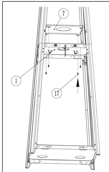
**23. Fix the plate cover(7) onto the middle plate(1) by screws(17).**
