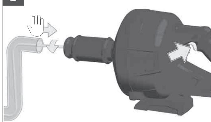
Switch on - cable rotates.
