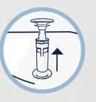
Lift the water trap from the waste outlet.
