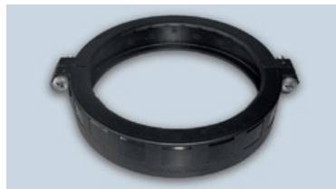
Brackets with dimensions equalling DN/OD 90 or larger are equipped with 2 screws. The maximum admissible torque is 7 Nm. (FIGURE 4)
