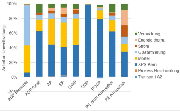
In most of the impact categories, the production of the XPS core is significant. The impacts are mainly caused by polystyrene, the input product. The energy used to manufacture the XPS core is also significant to a certain extent, especially in the categories of greenhouse gas (GWP) and acidification (AP) potential.
