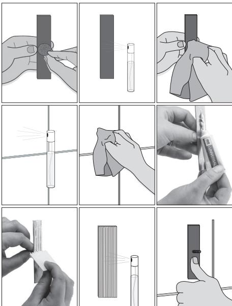
Pre-treat the surfaces of the plates and clean both the plates and the wall. Apply glue to the plates, spread out the glue and spray i.Cleaner onto the glue. Make sure the plates are attached to the wall!
