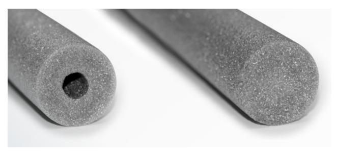
NOMATEC<sup>®</sup> Backer Rod Hollow & Full round profiles are manufactured from closed-cell polyethylene foam and are used as backing material for elastomeric and other cold-applied sealants. They are inserted into a joint to control the sealant depth and act as bond-breakers, without adhering to the sealant.
