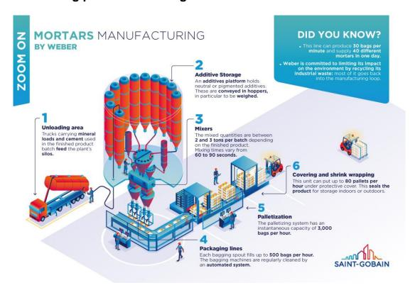
The manufacturing activities include grinding, drying, storing, mixing, packing and internal transportation. Packaging-related flows in the production process and all up-stream packaging are included in the manufacturing module, i.e., wooden pallets, bags, and LDPE film.
