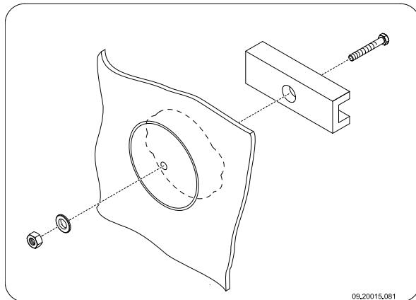
1. In the centre of the connection cover, drill a hole with a diameter of 10 mm.
