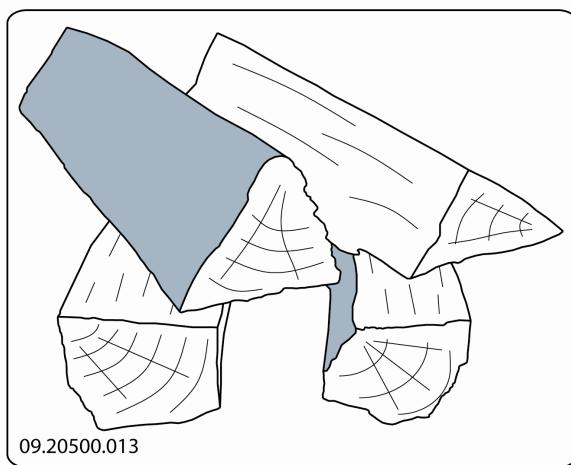
If the logs are stacked openly, the wood will burn quickly as the oxygen can reach each log easily. If you want to use the stove for a short while, make an open stack.
