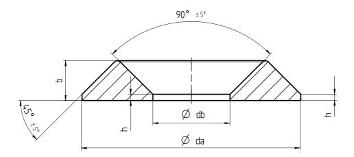
Washer for Power-Fast and construction screws
