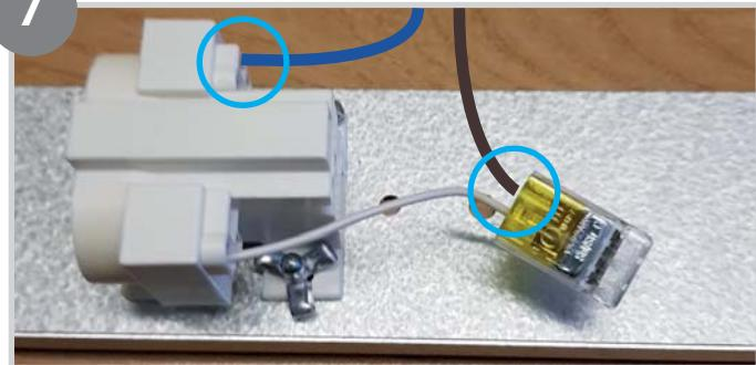
**EN** With this kit, the light source in your K2 is upgraded from compact fluorescent lamp (with electromagnetic ballast) to LED light source without ballast
