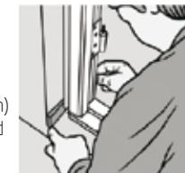
**EN:** Position frame in place according to predetermined position from (5). Wedge at the bottom of each side (opposing wedges from inside and outside) so top can be adjusted without bottom moving.
