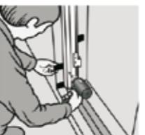
**EN:** Insert blocks to exactly fit at position of the frame fixing holes.
