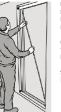
**EN:** Frame jambs must be square and plumb in both directions and the diagonals should be identical.
