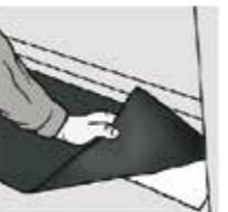
**EN:** If the base is of concrete a DPC must be placed under the whole length of the threshold.
