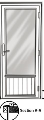
**EN:** Fit the door leaf into the frame and check the gap is even all around. Remove the wedges in top and bottom.
