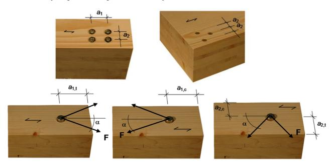
Definition of spacing, end and edge distances in the edge surface:
