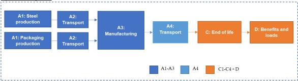
Steel and packaging materials are transported to a manufacturing plant where the galvanized timber connectors are manufactured. In this plant the steel is bent, cut and punched (all dry operations) to different shapes and sizes depending on which product that are manufactured. The connectors are then distributed to the final customers. After use the product is transported to waste processing, and the steel is recycled.
