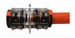
Make sure that the Microduct is correctly and fully inserted. The transparent body of the Connector allows a visual inspection of the correct and full insertion of the Microduct. Insertion of the Microduct into the Connector requires a moderate force. The Microduct and the Connector seal should not be scratched or damaged during the insertion, otherwise there may be leaks or further mis-functioning. Please, connect the Microduct by hand, without using any kind of tool.
