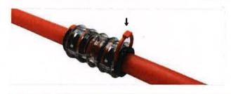
The Evolution NET.Fit products are pre-fitted with tamper proof locking clips as standard. If they have been removed, please replace with the correct locking clip after connecting the Microduct. The insertion of the locking clip between the Connector main body and the collet avoids any possible Mircroduct accidental disconnection.
