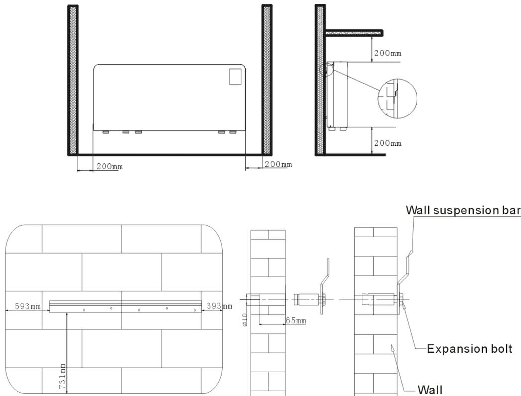
Using the enclosed, drill five holes for the wall mounting bracket and secure using the expansion bolts. When wall-mounting, the wall and the bracket level must be true or water will leak from the dehumidifier.
