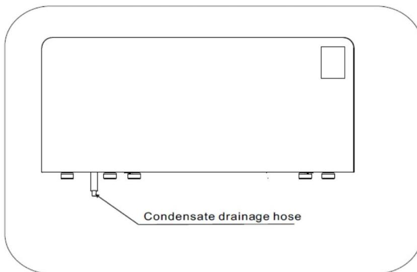
If you wish to move the drain to the other side, then you can do so by removing the side covers - **this should only be done by a qualified electrician and only when the units power supply has been turned off and isolated.**
