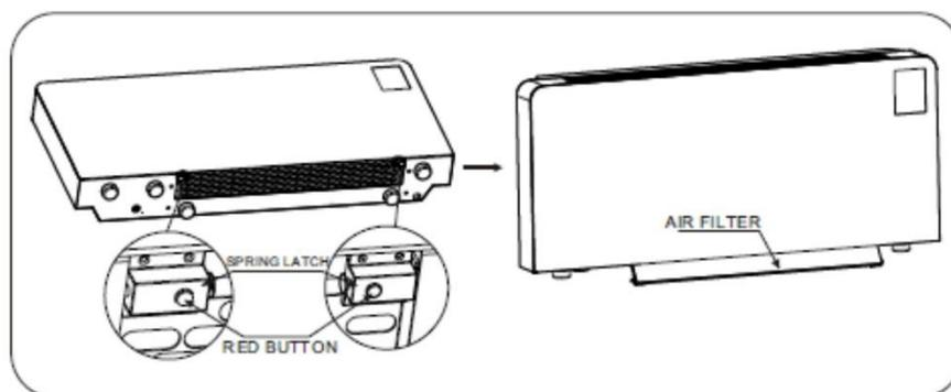
To remove the filter, press the two single red buttons to the left and right of the filter guard. This will allow the filter to drop down.
