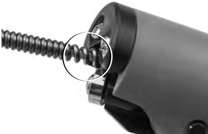
Figure 9 – Openings in Cable Wind at the End of Cable
