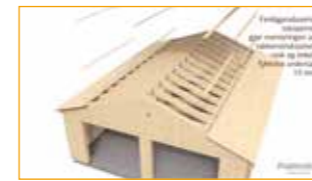
Monter undertak / rupanel
