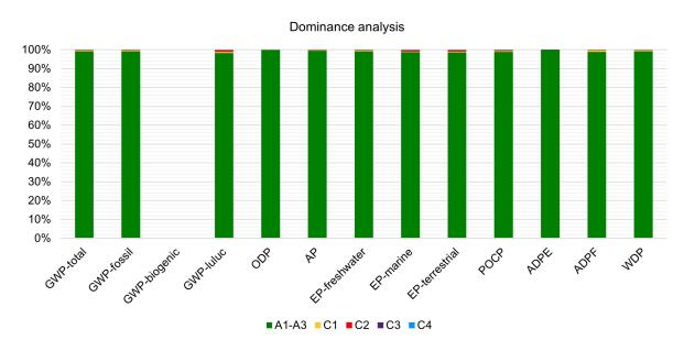
All indicators are significantly dominated by the production stage and the material and energy upstream chains (modules A1-A3). In modules A1-A3, stainless steel and energy consumption in particular contribute to the potential environmental impacts. Global warming potential fossil (GWP-fossil) is dominated by stainless steel (63 %) and electricity (25 %).
