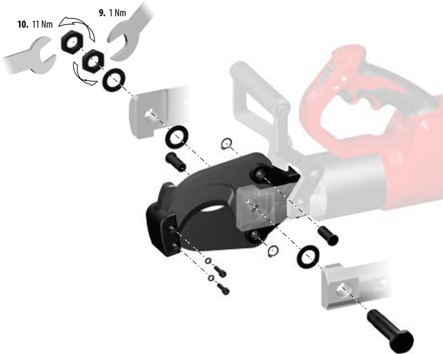
1. Use a wrench or pliers to remove the blade nuts and remove the blade bolt.
